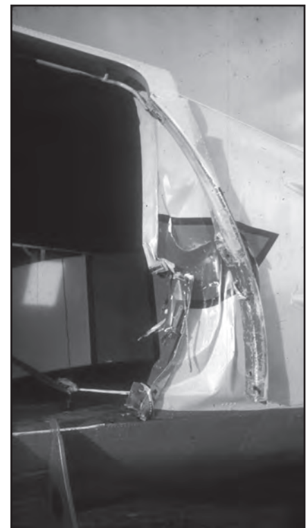
Door damage when Gene was sucked out of the aircraft.
